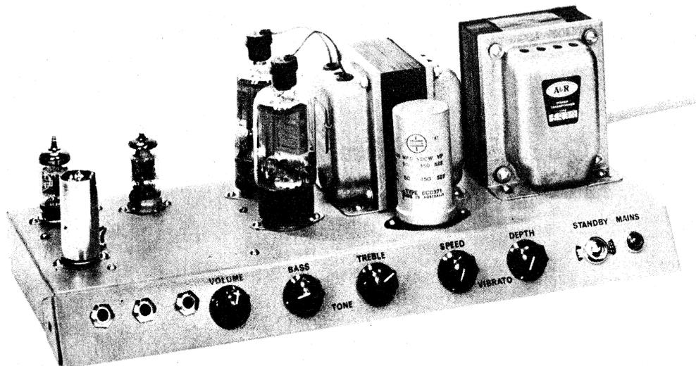
*From the front and from underneath, the 60-watt amplifier looks little different from the 40-watt version featured last month. Note the more elaborate input system.*
