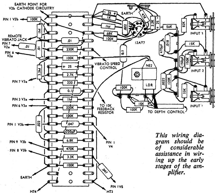
*This wiring diagram should be of considerable assistance in wiring up the early stages of the amplifier.*
