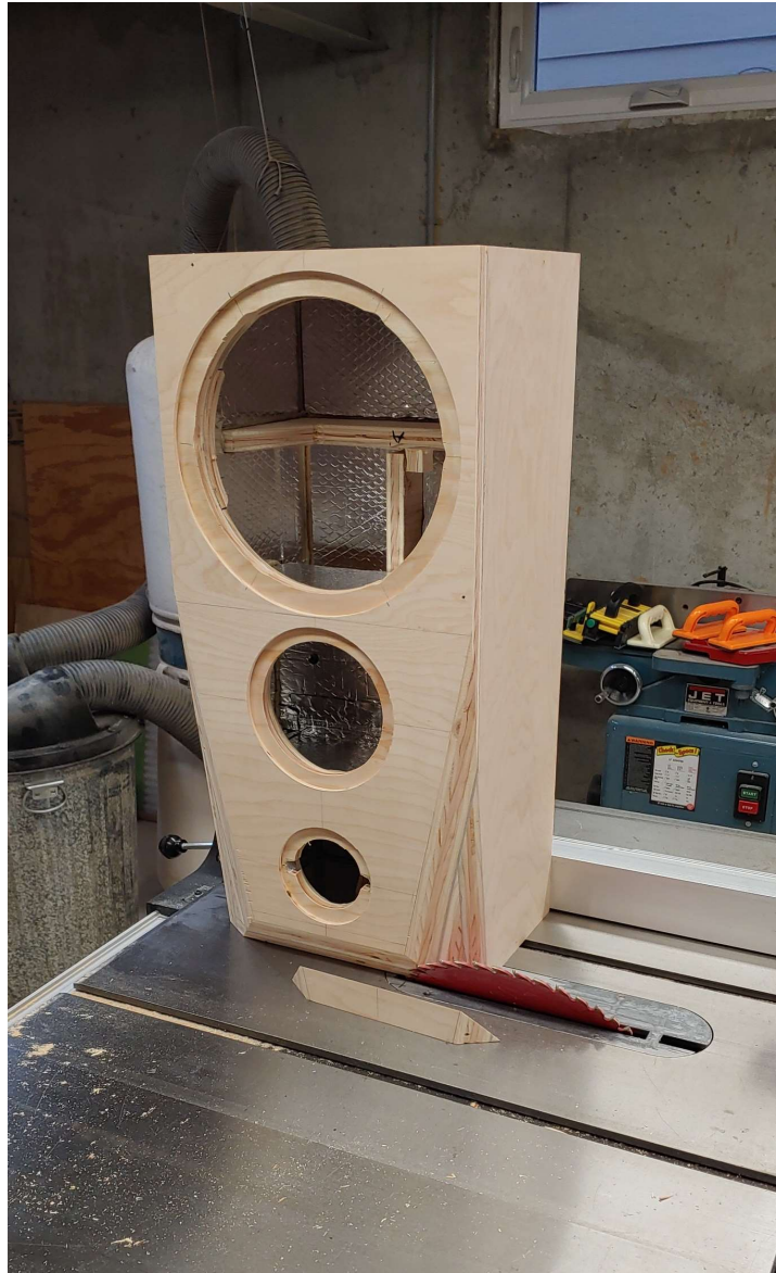
First cut of the top bevel
