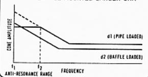
overlap the pipe fundamental resonance, so a limit must be placed on the maximum ratio of the two frequencies of about 1½:1.
