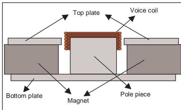
**Fig 1:** Cross section of a motor assembly
