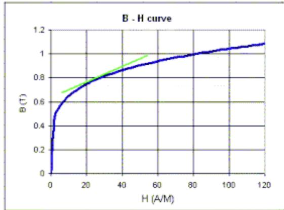
**Fig 5a:** An imaginary sample B-H curve
