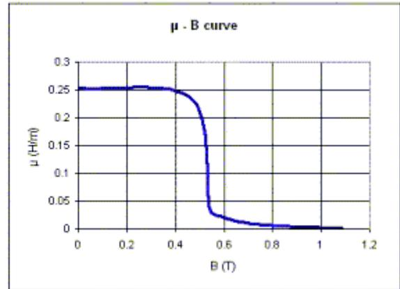
**Fig 5b:** Permeability ( $\mu$ ) - B curve
