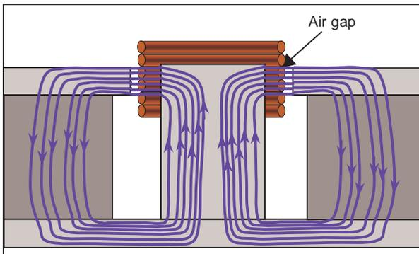
Fig 3: Static Magnetic fields in cross section view
