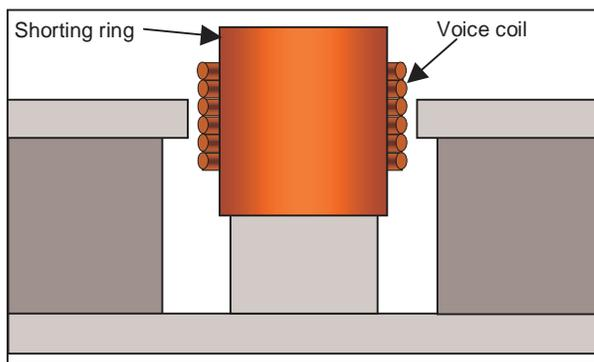
**Fig 6:** Shorting ring sleeve added to the motor
