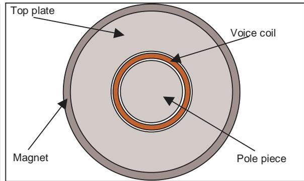
**Fig 2:** Top view of a motor assembly
