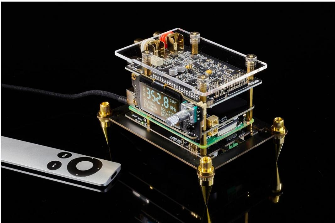
**5. Bast patternner of a FifoPiQ7 with the built-in FifoPi controller**
