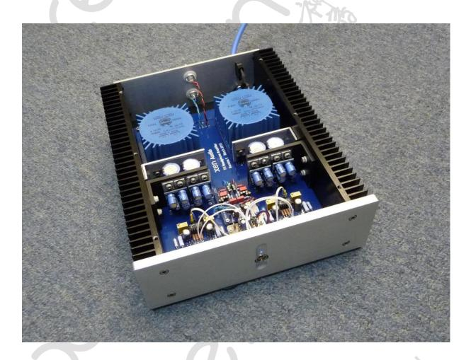
In the original F5-HA configuration, the RCA inputs were feed to a high impedance cross feed filter, followed by a JFET buffer. A volume control attenuator is placed between the buffer output and the F5-HA JFET input.
