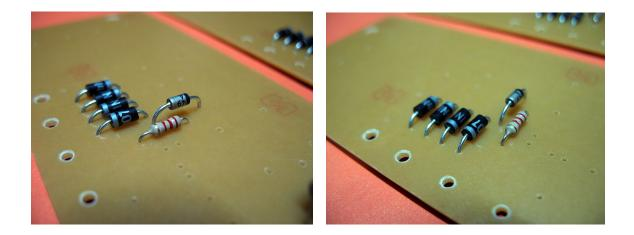
Install the four power resistors R15-R18. Since these resistors momentarily dissipate a huge amount of energy, it is wise to install them with a bit of clearance from the board to promote cooling.
