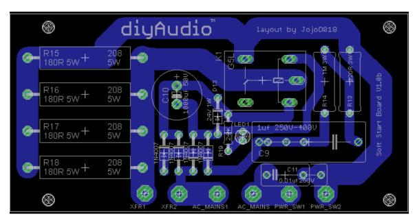
As a reference, the parts placement guide of the Soft Start board is shown below:
