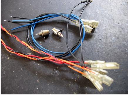
it's harder to dress a thick wire. AWG#16 stranded hookup wires at least. Of course no ones stopping you from using those ultra high end cables for wiring the amp. Use shielded wires for all small signal carrying wires.
