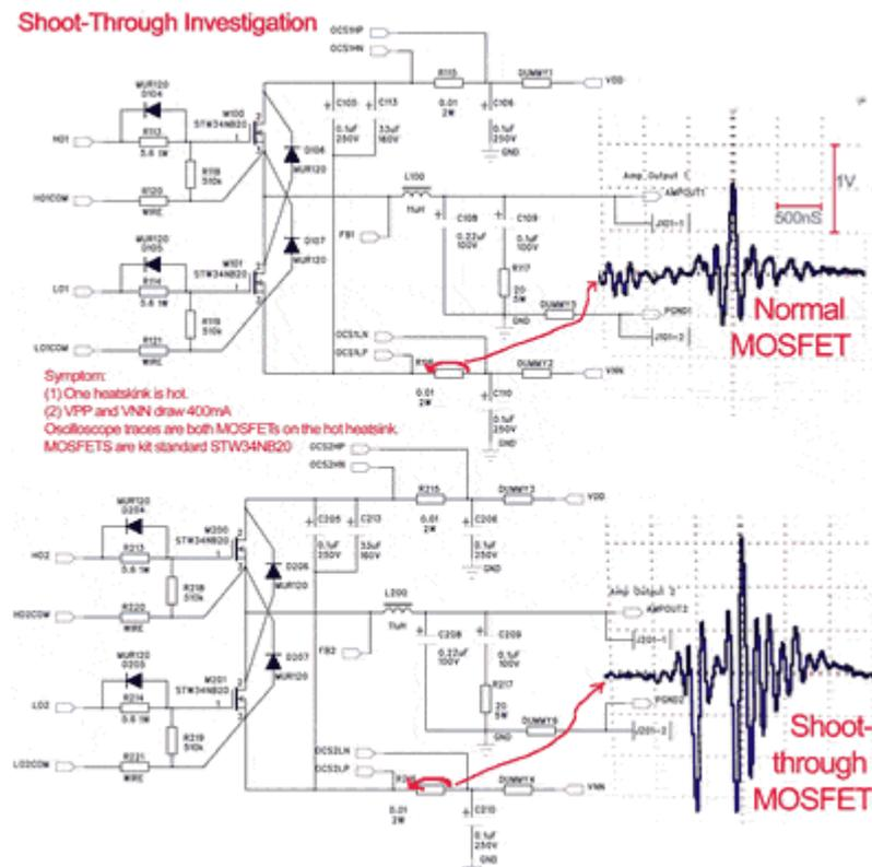
510k MOSFET gate pull down resistor (R118/218/119/219) is open circuit, eg from dry solder joint
