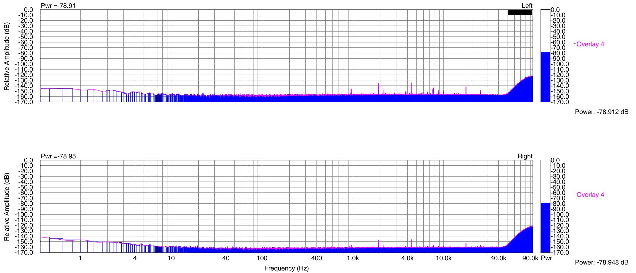
AA5381V1 ADC noise floor with input shorted to 50 Ohms. FS=192kHz, 0dB=Full Scale
