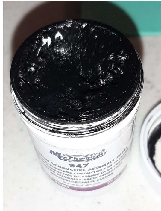
The Paste. It is about as “fun” to work with as wheel bearing grease. It contains carbon. I think they do not call it grease because it is not designed as a long-term lubricant.
