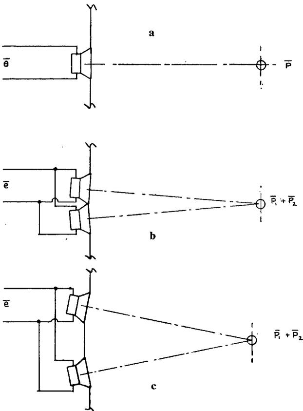
Fig. 2. Comparison of the performance of a, a single loudspeaker with b two such loudspeakers mounted very close together and c mounted several wavelengths apart.
