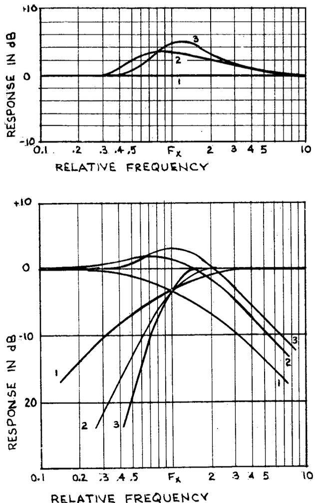
Fig. 3. Frequency response of asymmetrical constant-voltage crossover networks. a. In terms of power response as arithmetic sum of both channels. b. In terms of two channels independently [1].
