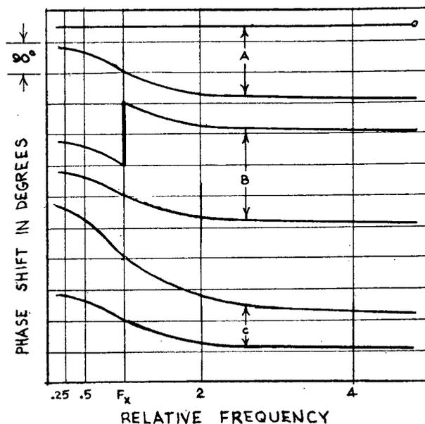
Fig. 4. Phase shift of summed outputs of constant-resistance networks. Lower curves show effect of phase reversal in one channel. a. First-order network. b. Second-order network. c. Third-order network.
