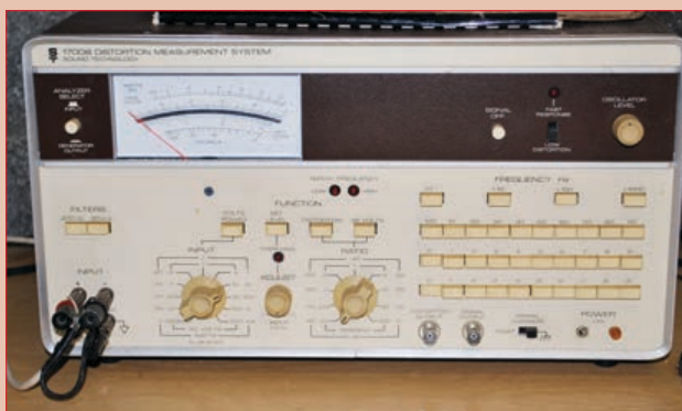
Photo 2: The Sound Technology 1700B test set was used for IC op-amp testing in the 1970s.
