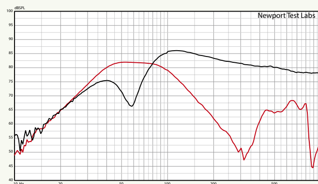
Graph 3. Low-frequency response of side-firing bass driver (black trace), and rear-firing bass reflex port (red trace). Nearfield acquisition. Port/woofer levels not compensated for differences in radiating areas. [Boenicke W5 SE Loudspeaker]
