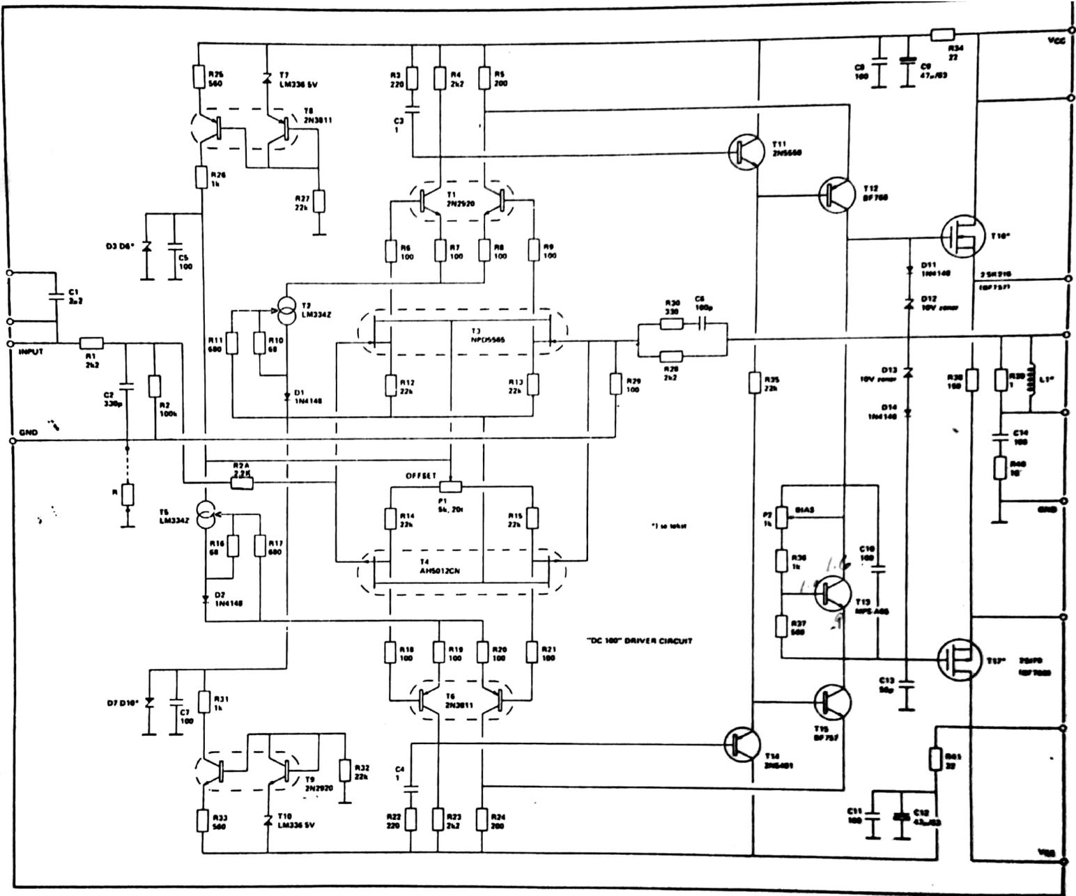
FIGURE 8: The complete DC 100 driver circuit. The output stage is the same as in the Servo 100.
