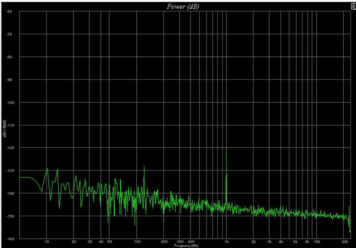
The 1Khz test signal is very easy to see in this spectrogram. We can see that the noise floor has moved up some also. This is the noise floor of the CCS. This shows that an ordinary PC sound card with a simple preamplifier and some good software can make some pretty low level measurements.
