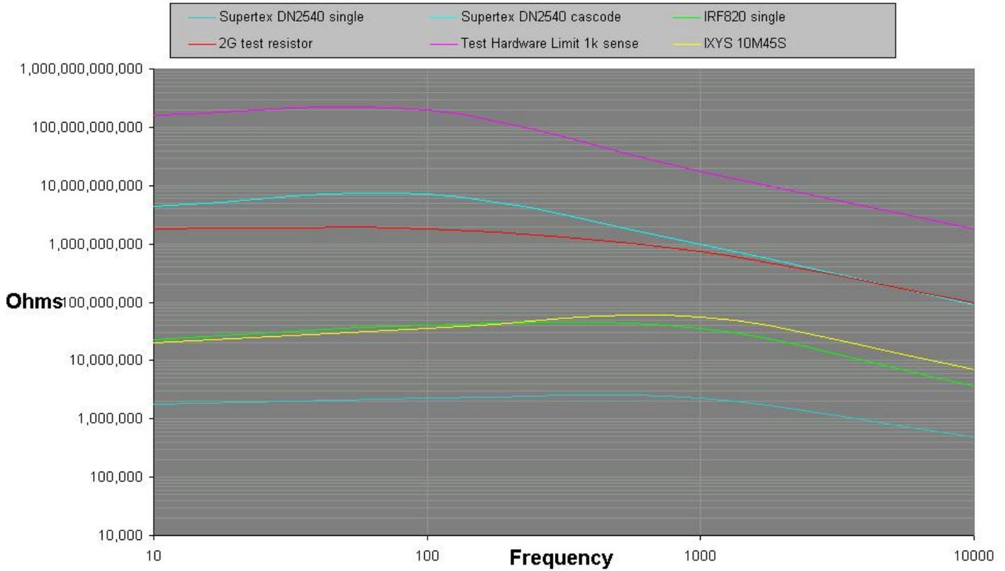
The Supertex parts are self biasing (depletion mode) mosfets. The single IRF820 mosfet was biased with a 9 volt battery. The IXYS 10M45S is an off the shelf 3 terminal CCS.
