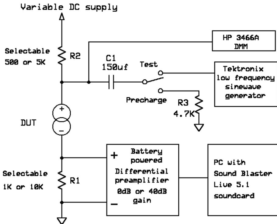
The basic test setup is to set the sinewave generator to 10Hz, 100Hz, 1Khz or 10Khz. For most testing the sinewave generator output is set to 10 volts RMS. On the higher performance CCS's at 10Hz the output of the sinewave generator is raised to 30 volts RMS. to make the test signal visible.
