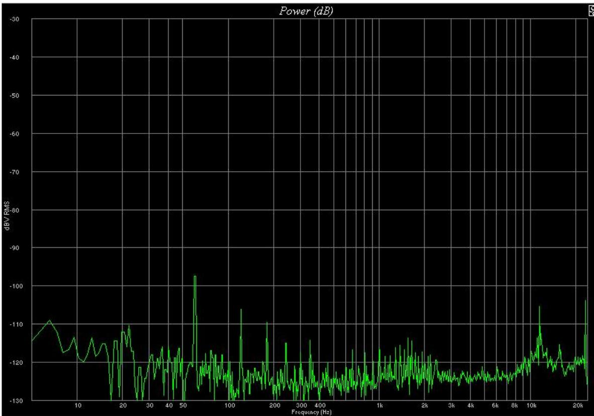
When the (-) input is opened the preamp makes a differential measurement. What this means is it only amplifies the signal difference between the inputs instead of the sum of the signal across the sense resistor plus the ground noise like in the SE case. It effectively ignores the ground loop noise that is common to both inputs. The next spectrogram shows the noise floor when making a differential measurement. Once again the sound card is the limiting factor.
