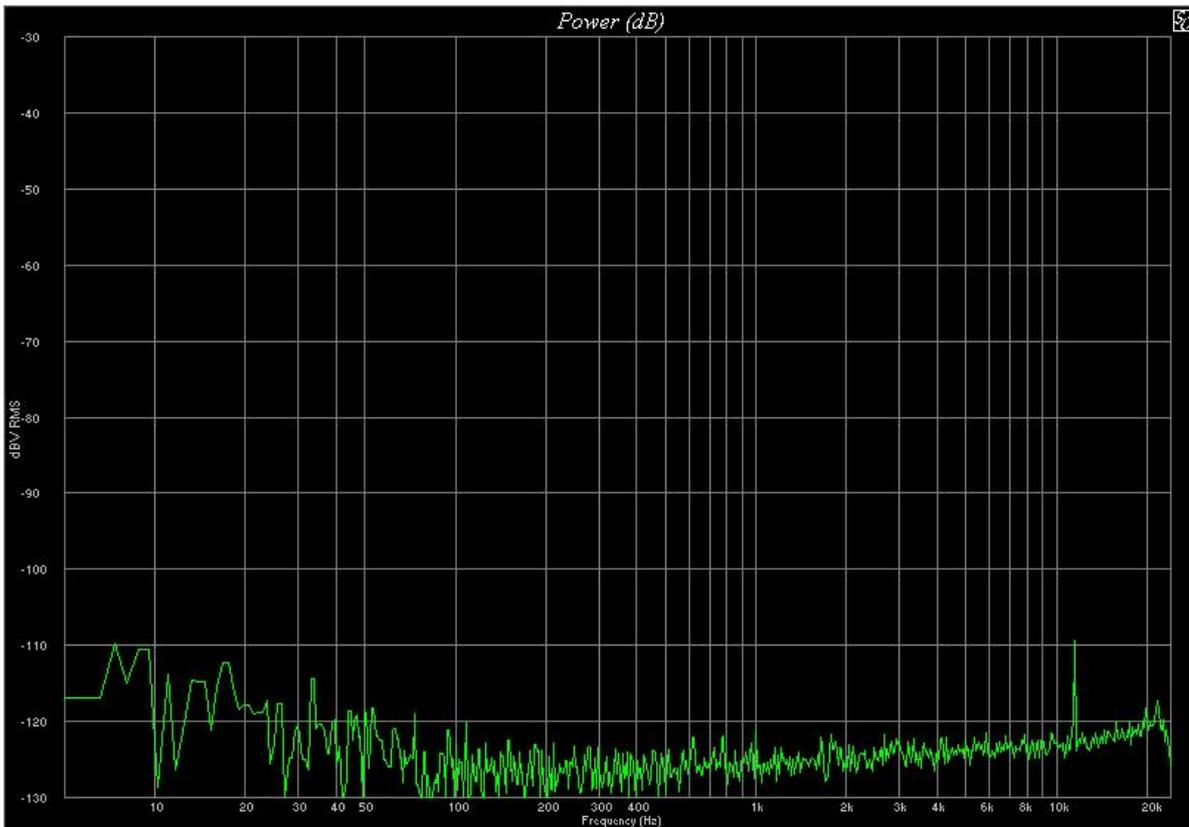
After setting the preamp gain to 40dB the test signal is very easy to see and measure. The tip of the 1Khz signal is still just below the -120dB line and you can see the 120Hz power line noise that was buried in the background noise without the extra gain.
