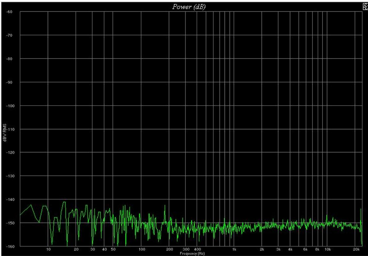
On to some real measurements. The next spectrogram shows the signal from applying 3 volts RMS. @ 1Khz to one of the new battery biased CCS's. The lower voltage drive is used to demonstrate the effectiveness of the preamp. In this image the 1Khz test signal is just barely visible in the "grass" of the background noise. The tip of the signal is just below the -120dB line.
