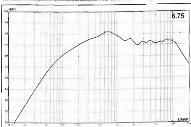
FIGURE 6.75: Frequency response for single 4.5" midrange at WTW center baffle location.
