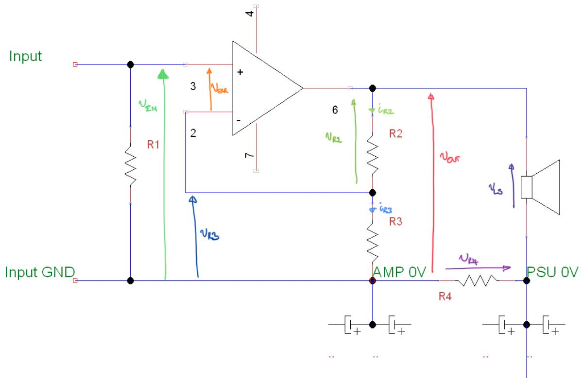
$$\text{NEGATIVE FEEDBACK} \Rightarrow V_{\text{err}} = 0 \Rightarrow V_{\text{in}} = V_{R3} \quad (1)$$
