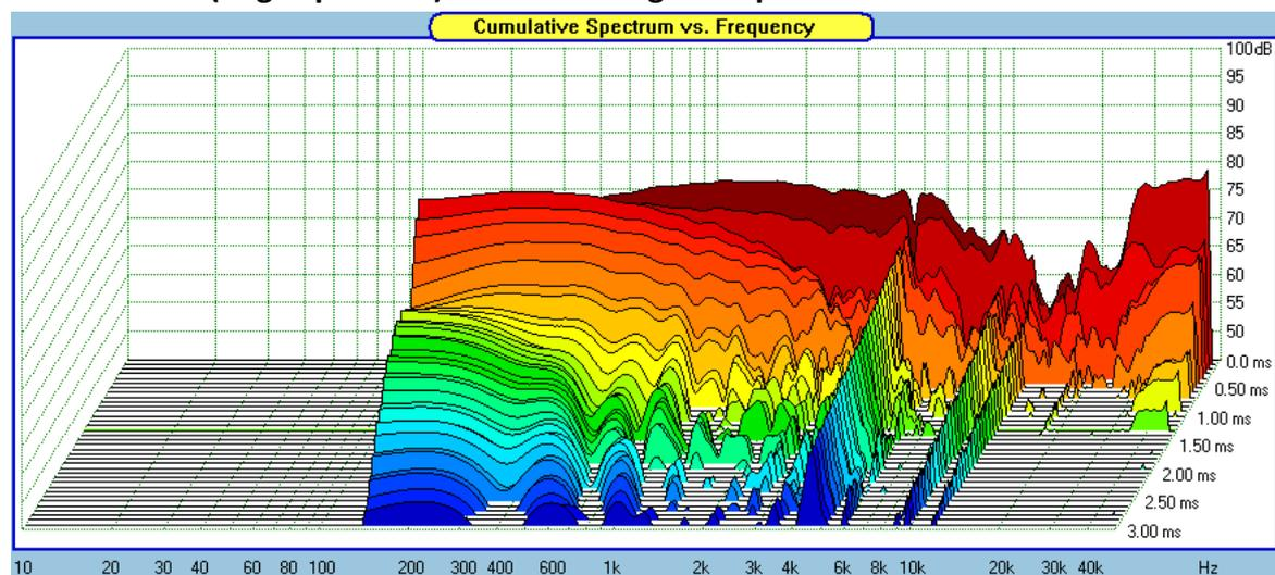
It is recommended that this driver is used from 500Hz up to approx. 4 KHz so it's a dedicated midrange and requires a very good high frequency to cover the top end.
