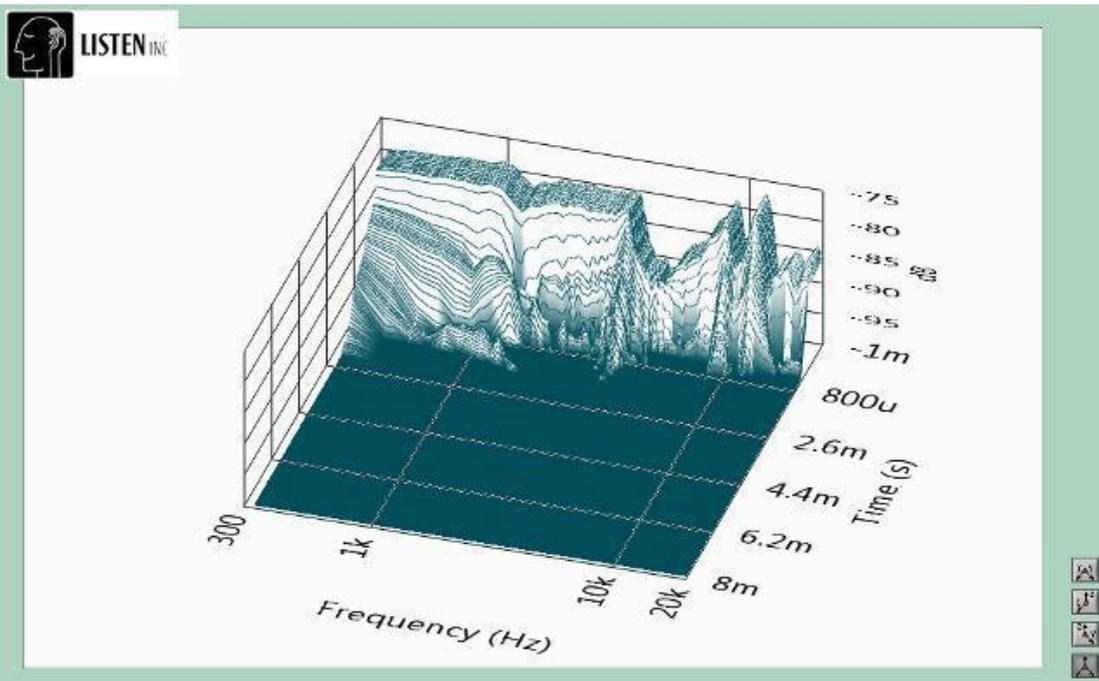
Looking at the energy decay performance there is not much to say....It is so clean with almost total energy decay in under 1ms....This is currently unmatched by any similar driver ( 4.5 inch wide band) in production today.
