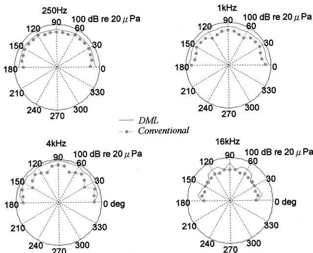
FIG. 13. Directional responses of the DML and the conventional speaker at 250, 1000, 4000, and 16 000 kHz, respectively. The radial scales are in dB with a full scale  $100\text{ dB re } 20\ \mu\text{Pa}$ .
