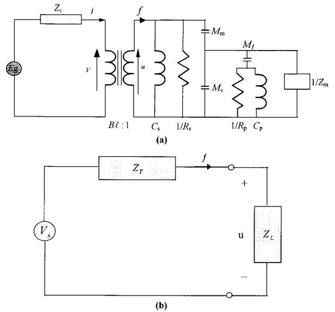
FIG. 4. Electro-mechanical analogy of a DML. (a) Equivalent circuit (mobility analogy); (b) simplified circuit. The symbols  $f$  and  $u$  in the figures denote, respectively, the force and the velocity of the panel.
