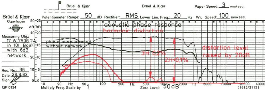
Noticeably low harmonic distortion. The unusually linear phase response is measured acoustically, not calculated!
