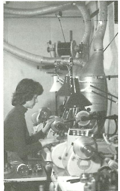
The voice coils are wound on high precision tools. Then they undergo special heat-treating process, after which a cross-section of the coil shows the honey comb configuration - the Hexacoil. In this forming process the wire and the bobbin are formed into an intimate and solid unit, which results in a compact and homogeneous coil / bobbin unit.
