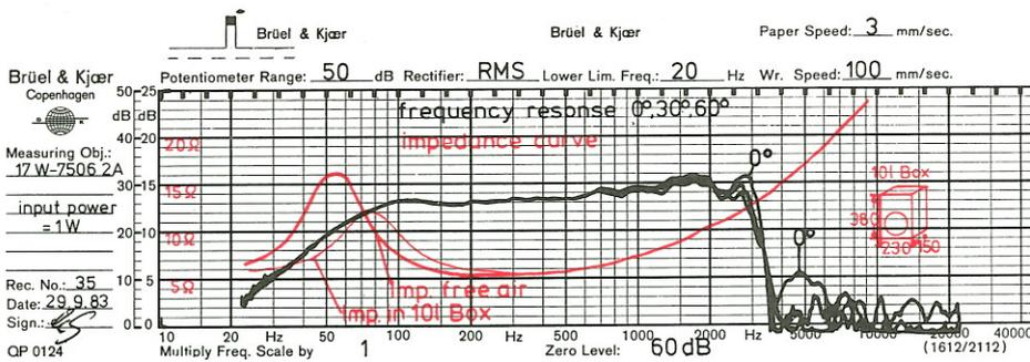
Frequency response flat to 2.5kHz, then rolls off smoothly. Obvious is similarity of curves at 0°, 30° and 60°, offaxis, especially in area above 1 kHz: no directional ambiguity. Impedance flattening with 24 uF, 6.7 ohms.
