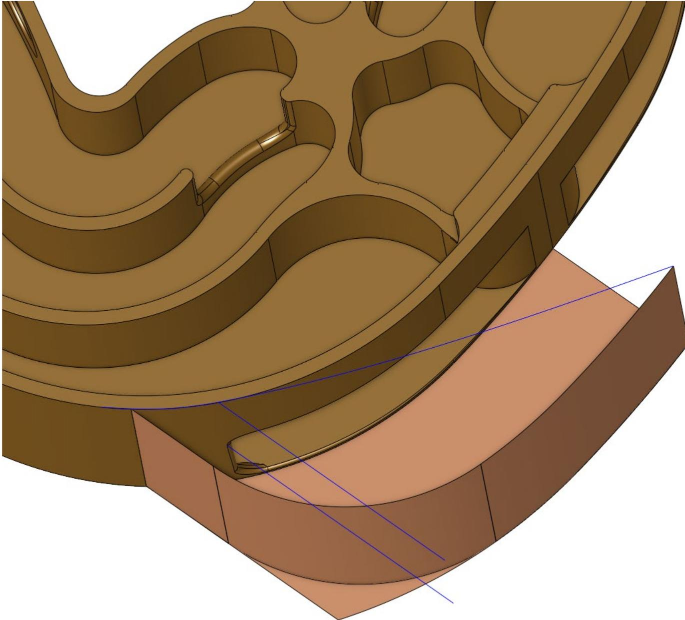
Considering horn directivity. Need to direct out and up. These simple surfaces are just a start, very basic. Need to add some contour and design the horn mouth with more exponential growth.
