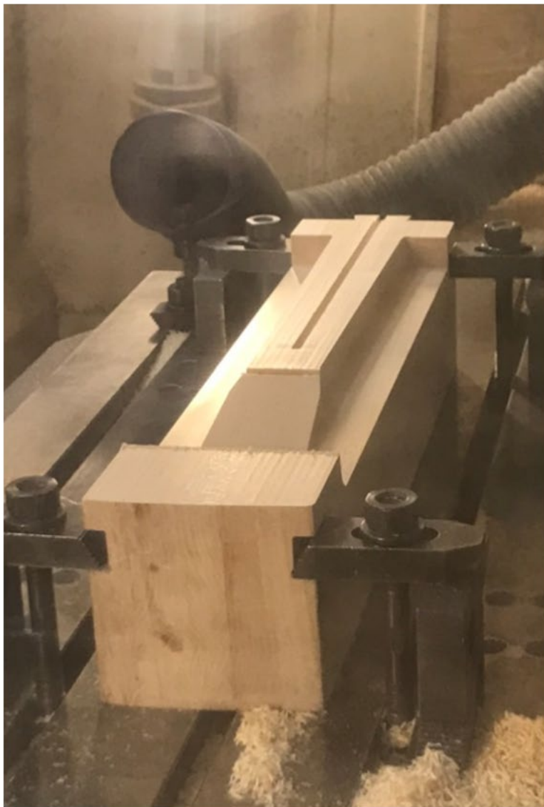
Solid stock on the CNC machine.
