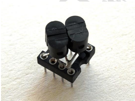
Figure 1 Dual Source Follower with TO92 N-JFETs on DIP8 header
