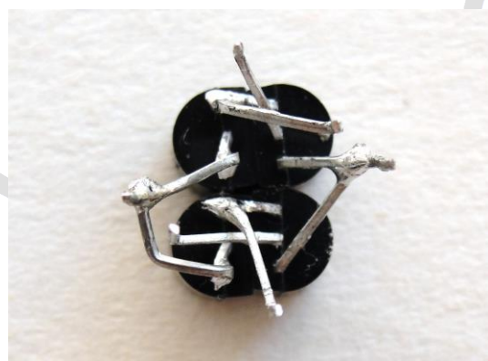
Figure 1 Dual Source Follower with TO92 N-JFETs on DIP8 header
