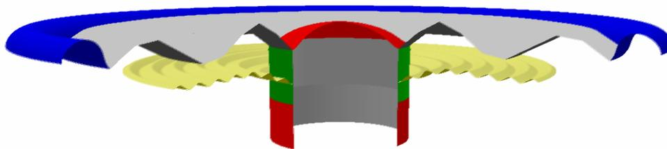
Figure 2. 3D plot of Mode @ 2868 Hz
