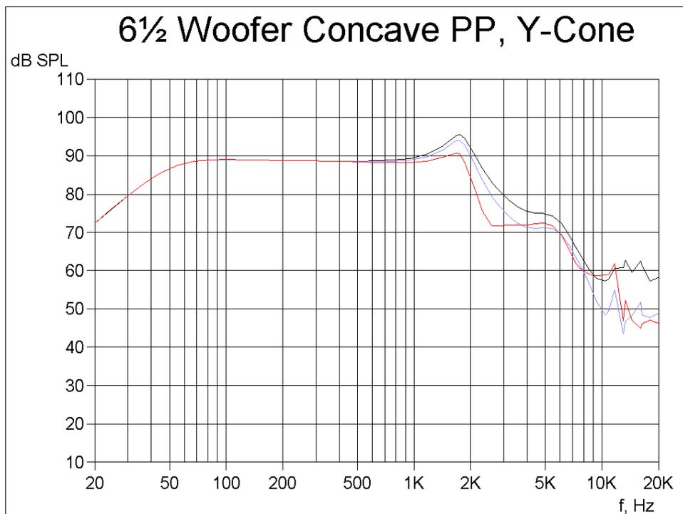
Figure 12. Response of concave curved PP-cone with bended cone neck (Y-cone). The response shape is approximately 2<sup>nd</sup> order Low Pass.
