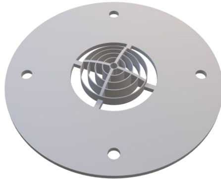
Figure 5: 3D print file of Phase Plug Extension
