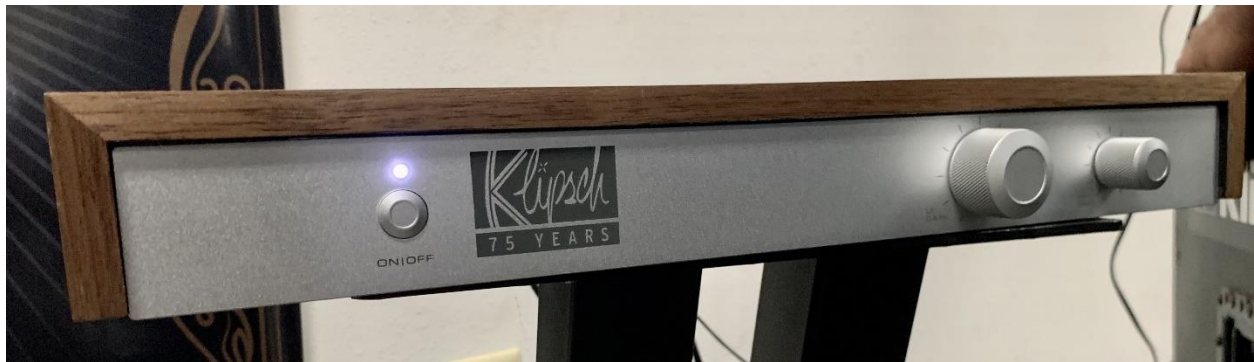
Figure 15: Klipsch-provided fixed DSP crossover for second-gen Jubilee
