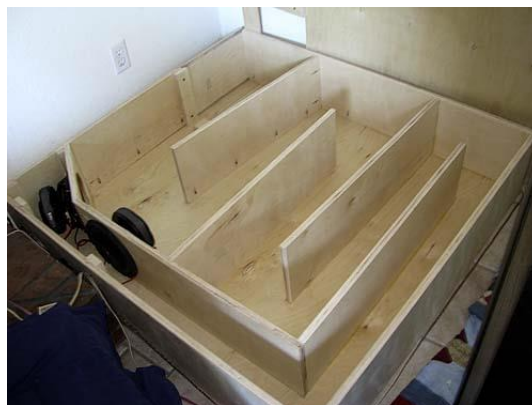
Figure 12 DIY TH-SPUD on floor with side removed showing drivers, baffles, and horn mouth
