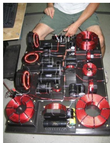
Figure 2 A single passive first gen Jubilee crossover
