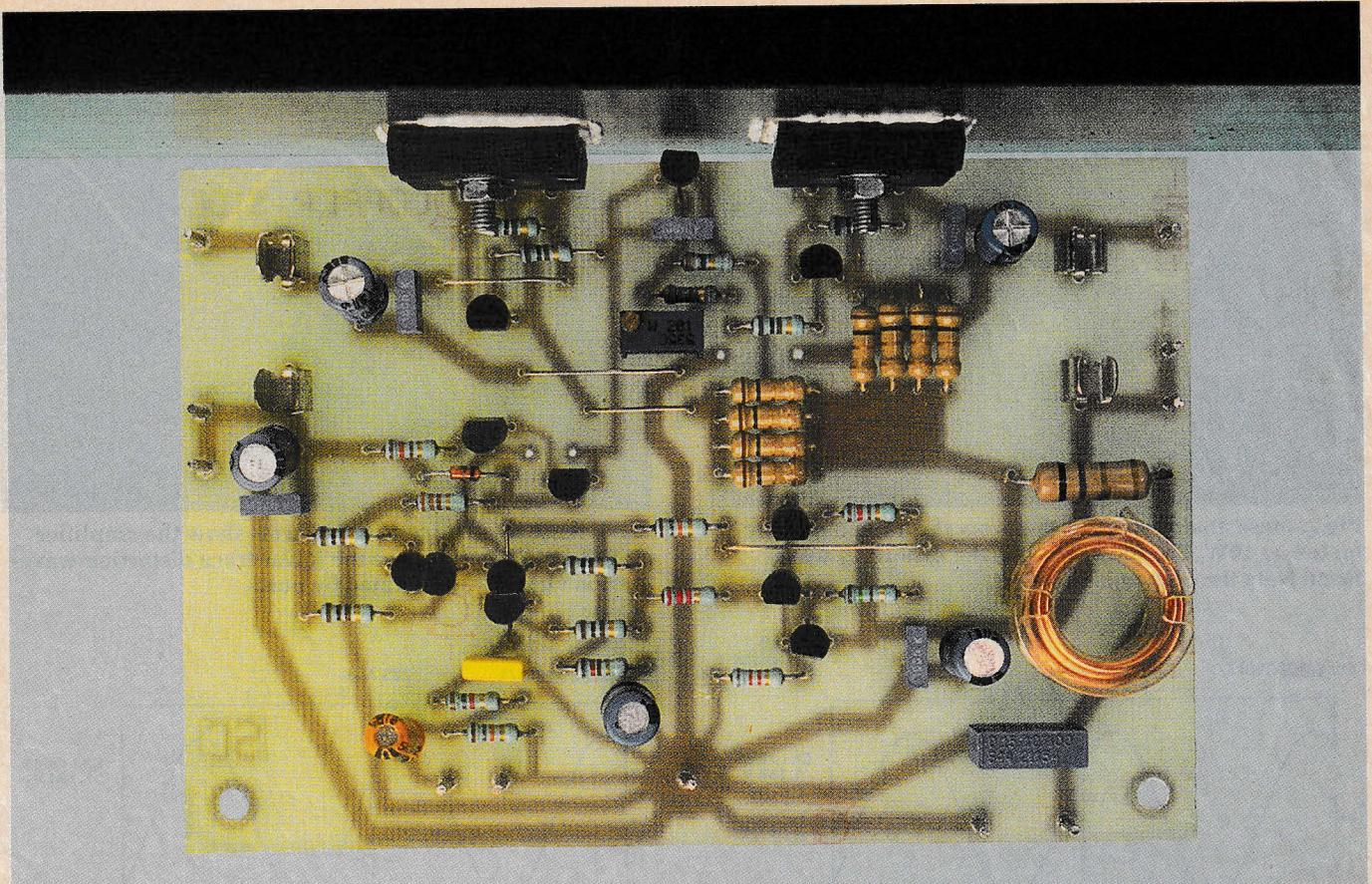
The PCB design is critical to the performance of the amplifier so don't alter it in any way. Note that two pairs of transistors (Q1 & Q2 and Q5 & Q6) are thermally coupled together and don't forget to fit flag heatsinks (not shown here) to Q11 and Q13.
