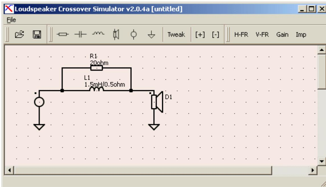
Each time your circuit is electrically valid, the simulation will show all the current results in separated windows. You can open these windows by pressing "H-FR", "V-FR" ... buttons on the toolbar.
