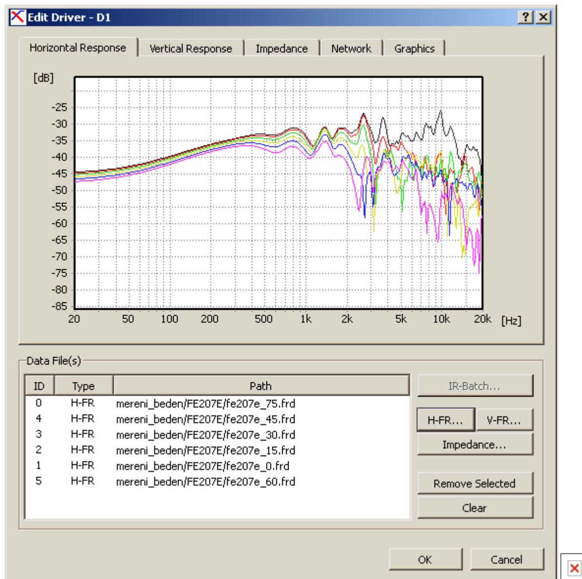
**Naming convention** for data files is as follows: frequency response file name **must end with a number** (to one optional decimal place, e.g. "tweeter\_22,5.txt"). This number (and only this number) gives information about which angle from axis it was measured for. Even if you load only one file (for example on-axis only), you still must end it with some number ("tweeter\_0.txt").
