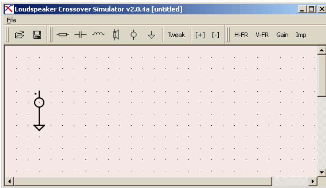
2) Add a driver to the circuit via "Add Driver" toolbar button. Enter a name for the driver when asked.
