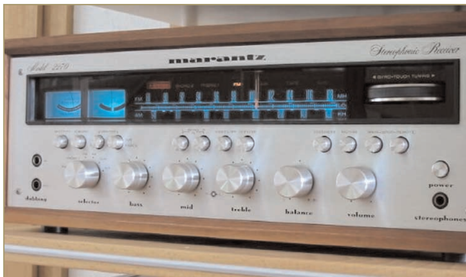
The Marantz 2270 Receiver. The model numbers of the “2200” series receivers included power ratings. In this case, power output was 70 watts per channel.
