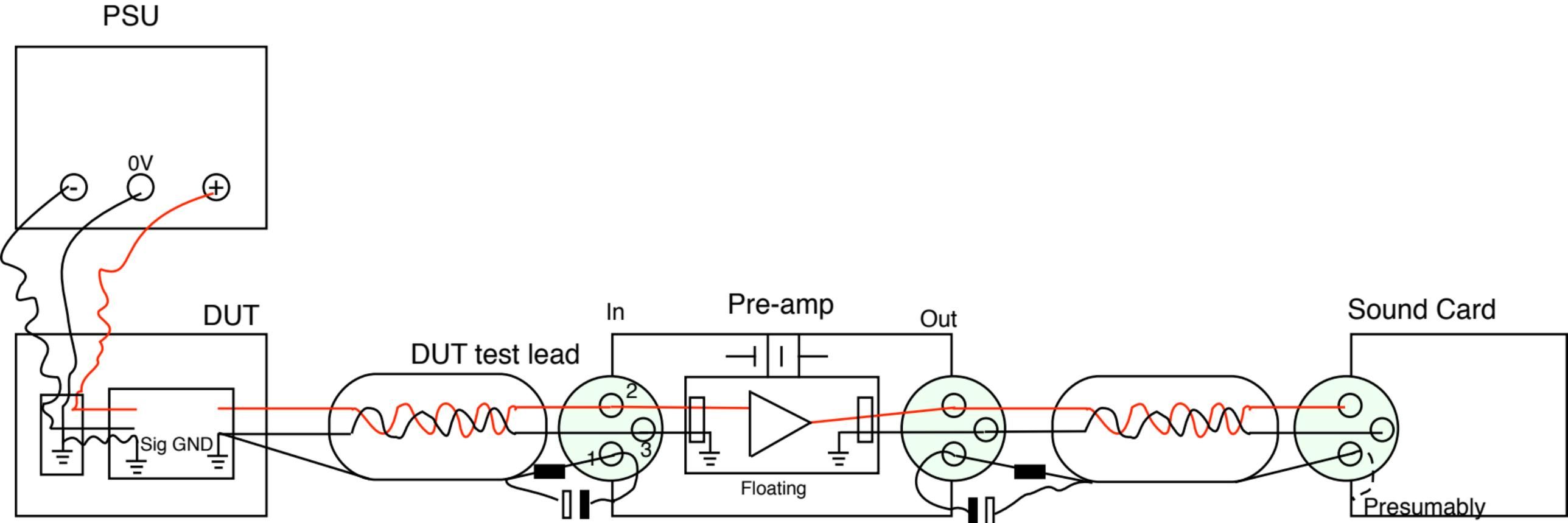
DUT has separate power and signal ground
