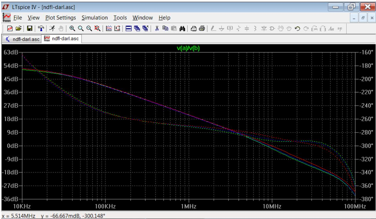
Total loop gain around OPS, with additionally engaged intermediate stage:
