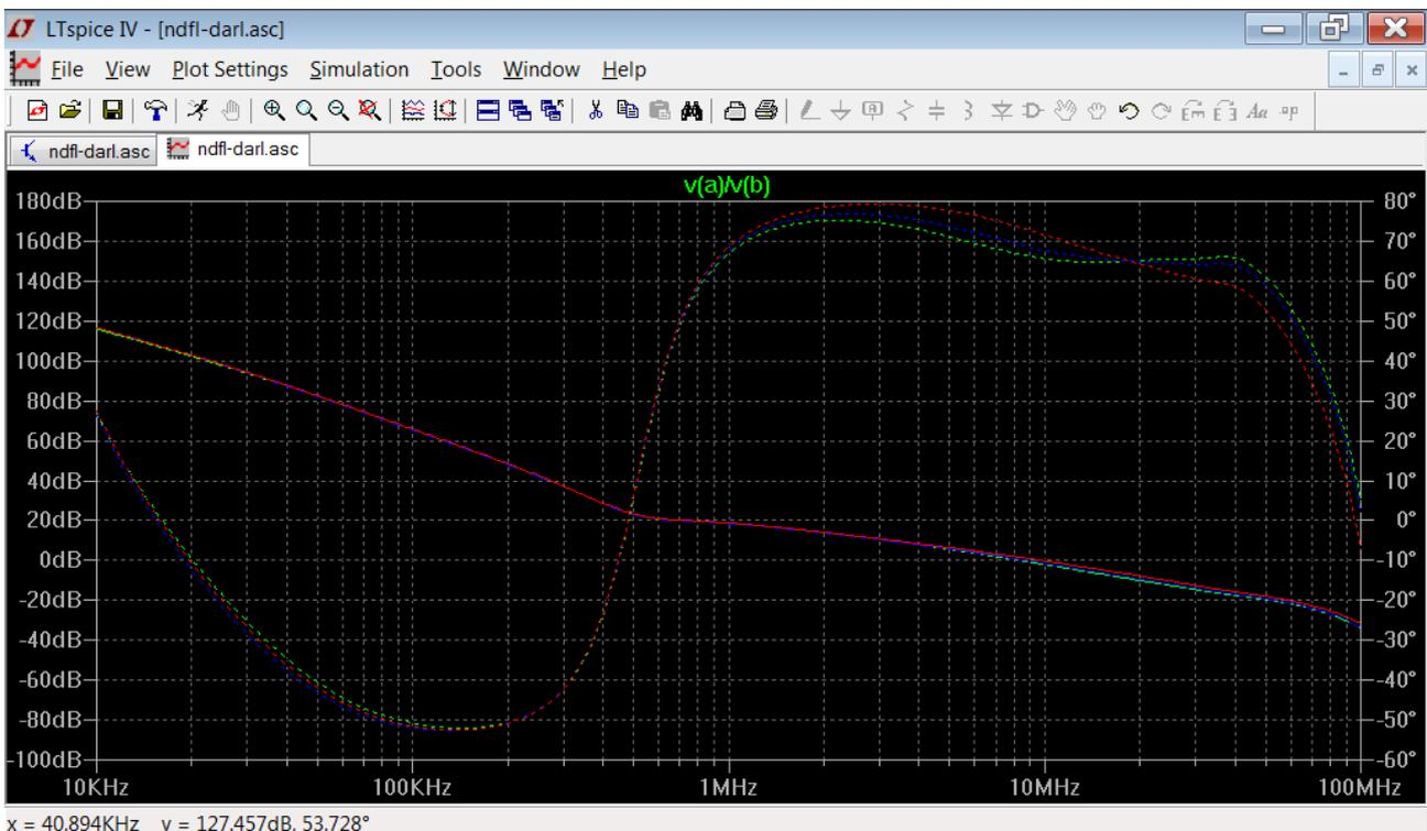
Loop gain in intermediate loop, global loop not active:
