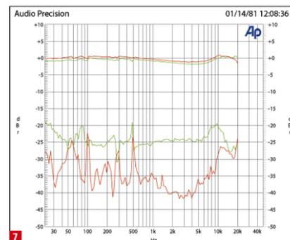
wer, red curve shows the crosstalk from the left to the right channel. A second test also measures the frequency response of the right channel (red, above) and its crosstalk on the left channel (green, below).
