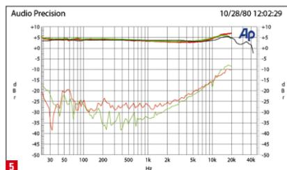
**CARTRIDGE:** The frequency response shows how balanced the cartridge reproduces all frequencies, the crosstalk (lower curve) shows mutual influence of the channels.
