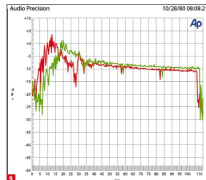
**TYPICAL:** In tangential arms, the mass is often greater for horizontal (red) than for vertical (green) movements, leading to different resonance frequencies.
