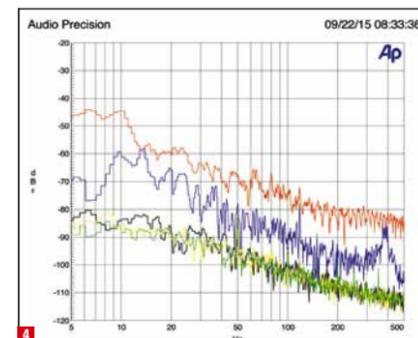
**DISTURBANCE:** The rumble spectrum unmistakably shows self noise of the turntable.
