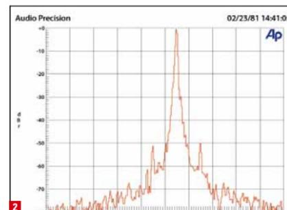
**FLAWED:** This turntable shows a deviation of the nominal rotational speed as well as strong, partly periodic fluctuations.
