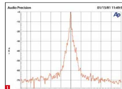
**HITTING THE MARK:** This turntable complies exactly with the nominal rotational speed, short term fluctuations are irregular and high.
