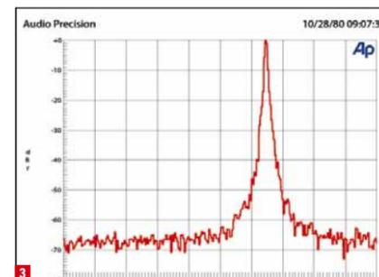
**FEW FLUCTUATIONS:** The sharp tip shows that the average speed hardly varies, but differs significantly from the target value.
