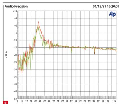
**GOOD COMBINATION:** In this cartridge tonearm combination, the lateral and vertical bass response resonance are nearly ideal at 9 Hz.
