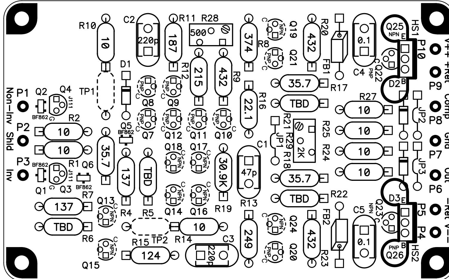
PARTS LOCATIONS FOR TRANSISTORS WITH CBE PINOUT
