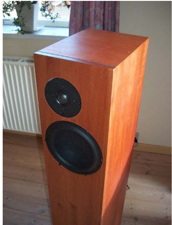
2.5 clone with ScanSpeak D2905-9500 tweeter.
