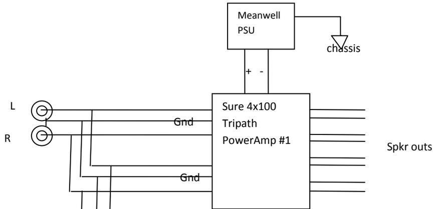
Now I add a second Power amp board so I can have 4 stereo zones. It has its own Meanwell PSU.
