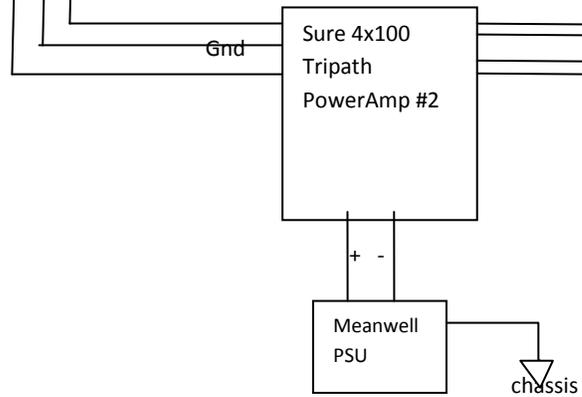
I probably have some feedback (ground) loop causing this. I tried creating a local grounding point (not connected to the chassis) to which I connected the Gnds of the two amp boards and the input ground. It didn't help.
