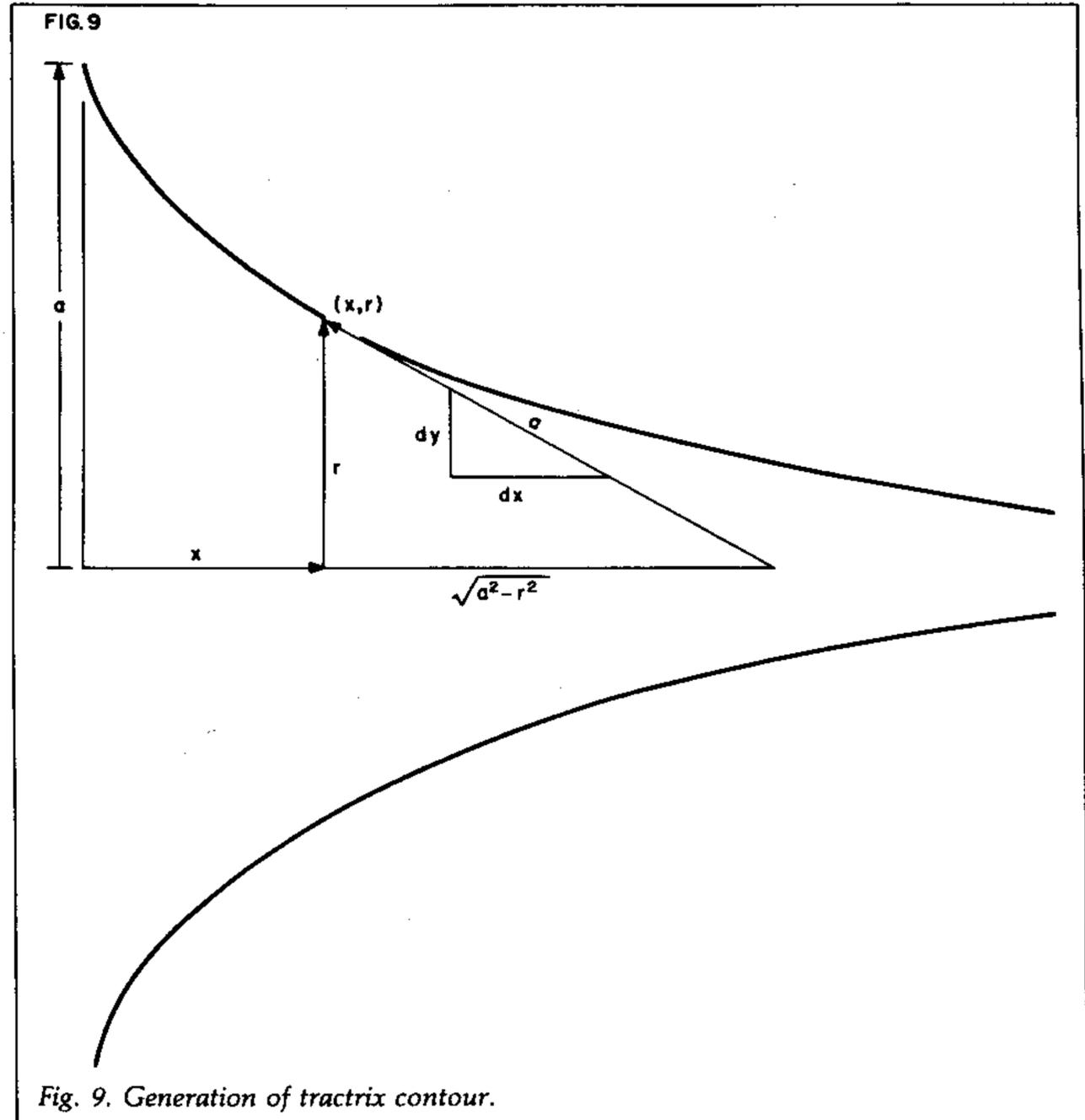
Fig. 9. Generation of tractrix contour.
