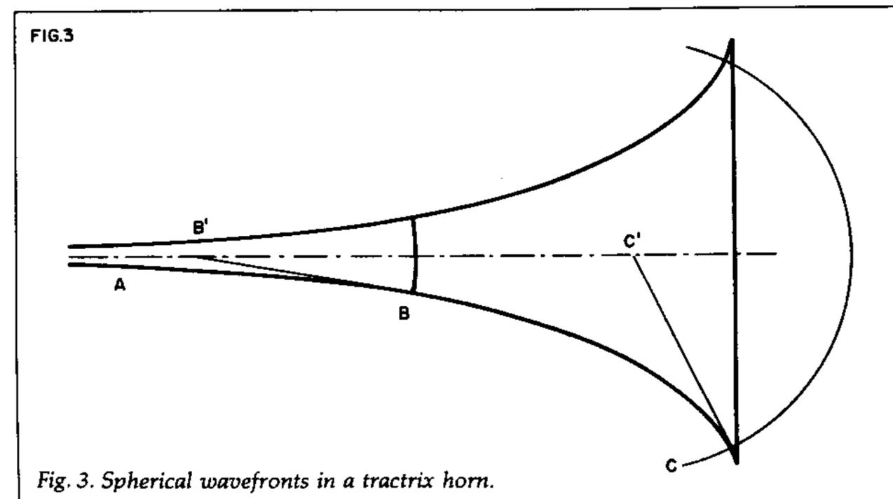
Fig. 3. Spherical wavefronts in a tractrix horn.
