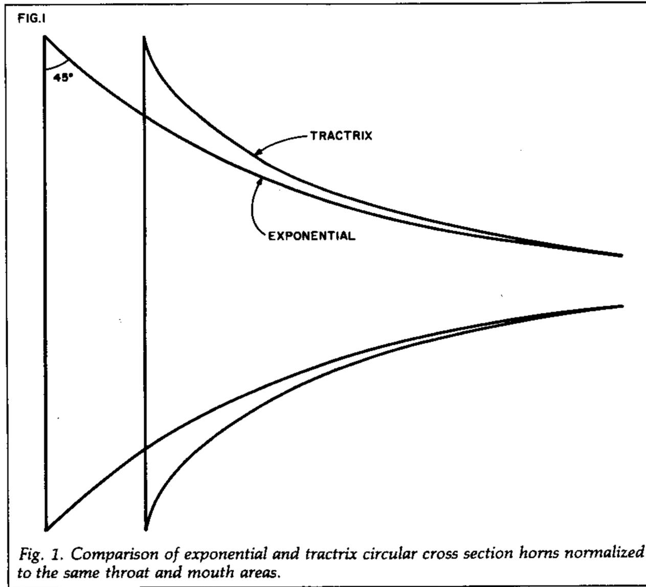
Fig. 1. Comparison of exponential and tractrix circular cross section horns normalized to the same throat and mouth areas.
