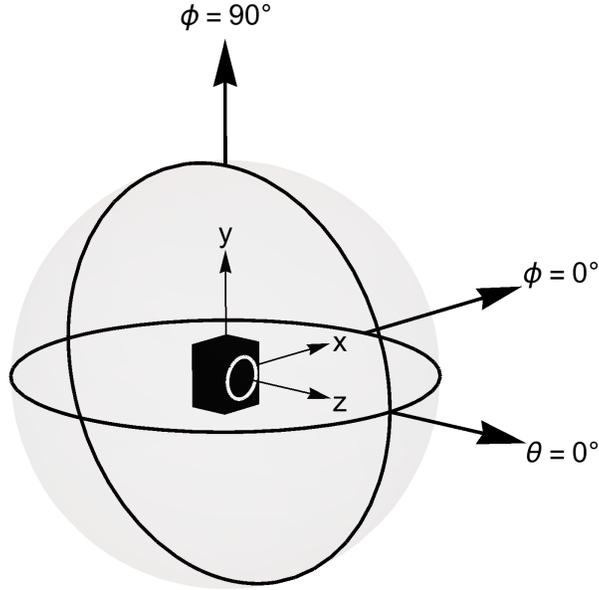
Figure 1: Diagram of the coordinate system. The reference axis ( $\theta = 0$ ) passes through the center of the (upright) loudspeaker cabinet, parallel to the ground. The two circles represent the horizontal and vertical measurement orbits.
