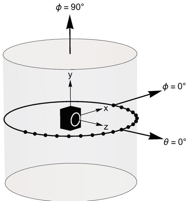
Figure 7: Diagram of single-half-plane measurements.
