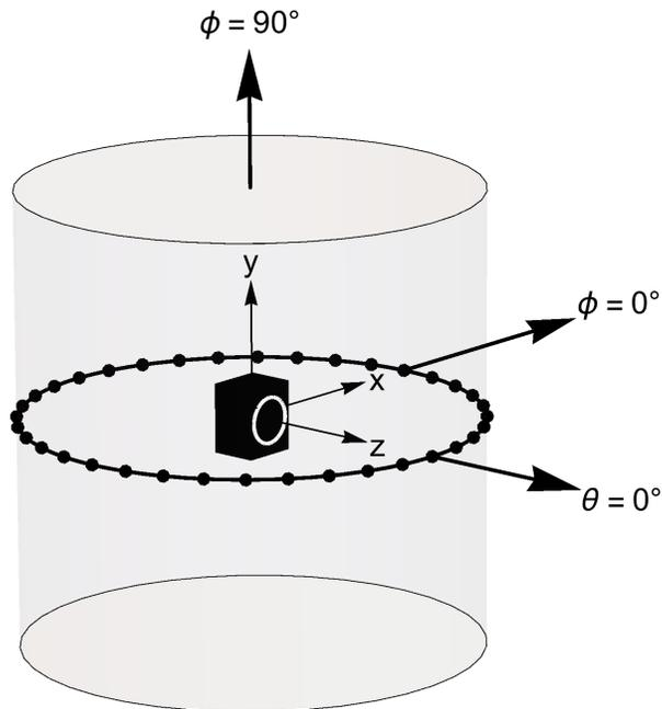
Figure 5: Diagram of single-plane measurements.
